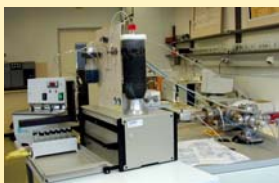
Figure 2. SPINMAS coupling with automatic sample changer and quadrupole mass spectrometer
