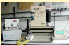
Figure 1. SPINMAS automatic coupling with sample changes
