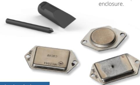
Two examples for different piercing devices used in quality control of electronic device packaging applications. The piercing devices can easily puncture electronic device packages to release the filling gas.
