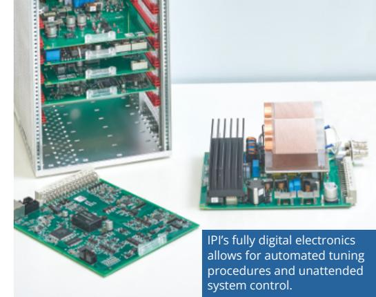
IPI's fully digital electronics allows for automated tuning procedures and unattended system control.
