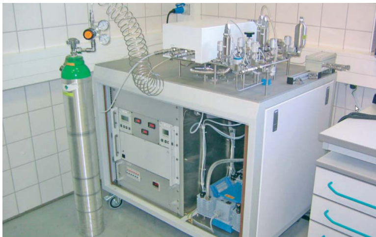
The GAM 400 mass spectrometer, here with different inlet systems, serves a mass range of 1 to 300 amu.
