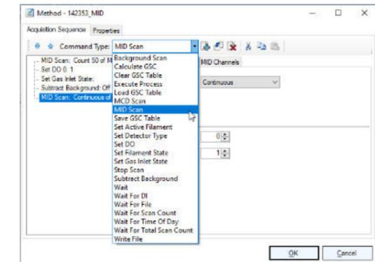
IPI ProxiMass System Control and Automation Software allows the definition of complex methods to automate experimental procedures.
