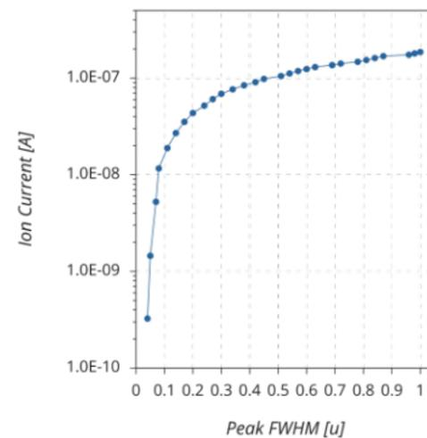
The resolution value of a quadrupole mass spectrometer is one of the most important performance indicators. The resolution defines the capability of a spectrometer for a specific application or to perform a specific measurement task. The EDA407 offers class leading analytical performance also in this respect with a resolution of 280 at m/z 28.
