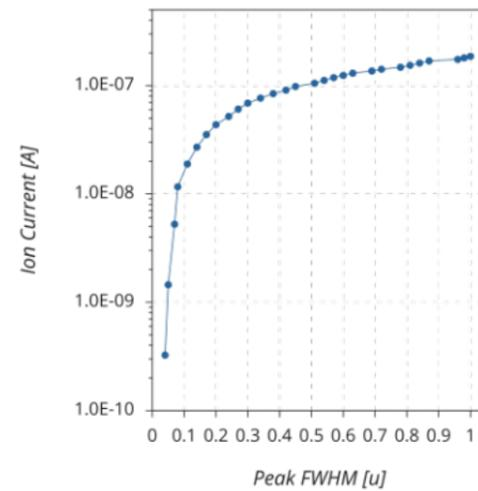
Fig. 4 (left): Strongly reduced Zero Blast below  $m/z1.5$  suitable for applications in hydrogen related research.
