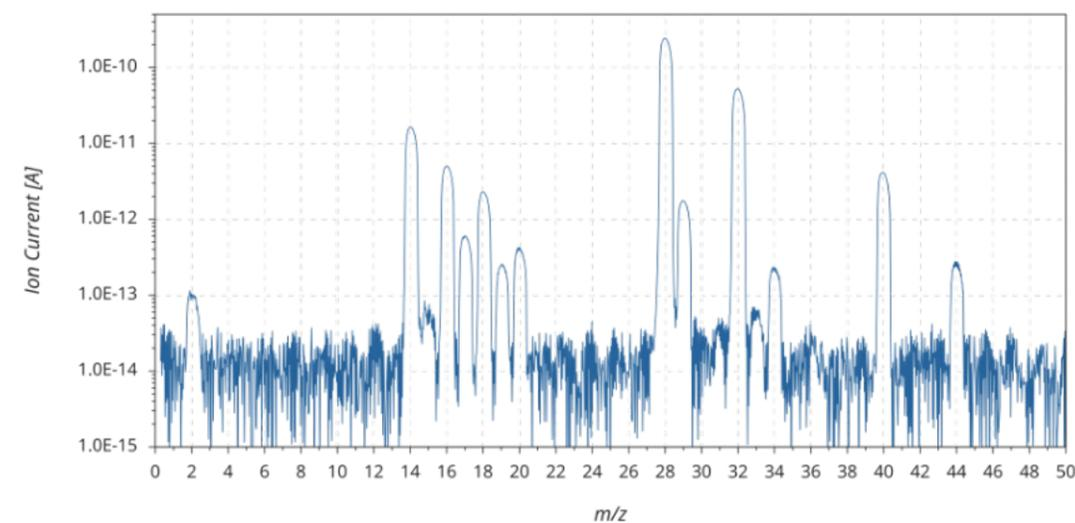
Fig 1: Mass spectrum of ambient air recorded with the system's Faraday detector.
