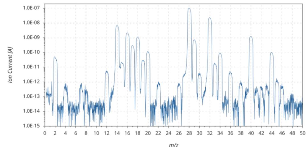
Fig 2: Mass spectrum of ambient air recorded with the system's secondary electron multiplier (SEM).
